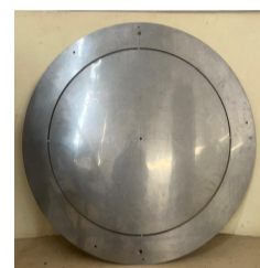
Annular mask at the telescope entrance: Outer diameter: 738 mm Inner diameter: 728 mm Width of the annulus: 10 mm
