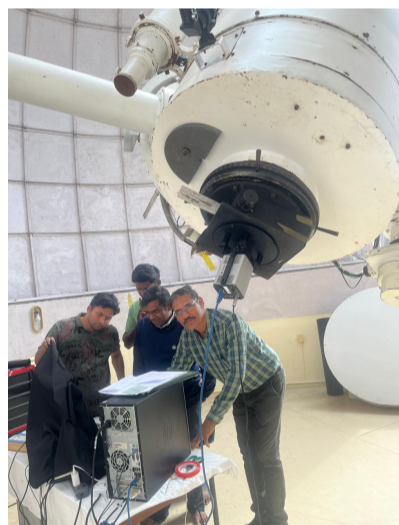
Re-imaging unit with Andor Zyla 5.5 camera. Cassegrain focus image was re-imaged with a magnification of about 1.92.
